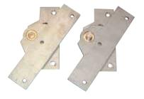
Please note that the actual opening (C) is smaller than the total door size (O) due to the pivoting mechanism. The position of the pivot system will in turn depend on the total load of the louvre door. Renson® can assist you in determining the correct sizes.
